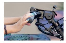
The quadriplegic version includes a **handlebar without** levers for smooth movements when braking and accelerating.
