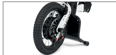
16" wheel, ultra-grip tyre and aluminium double-wall rim.
