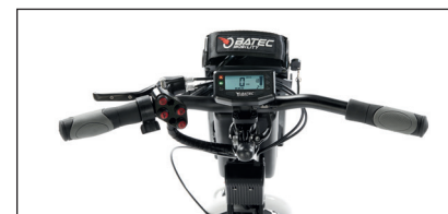
Handlebar option with right or left throttle and Monolever brakes for hemiplegics.
