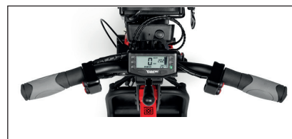
G&B handlebar option without levers for quadriplegics.
