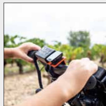
Gas & Brake handlebar without levers *: lets you accelerate and brake with gentle movements of the handlebar.
