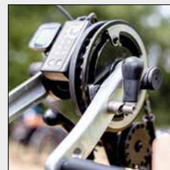
BATEC MAGIC LEVER crank arm release system (Pat. Pend.)***: with assisted starting mode so Batec users can enjoy the zero-effort mode.
