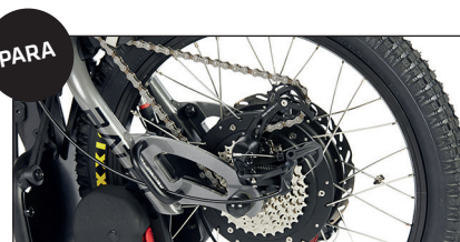
9-pinion gear change.
