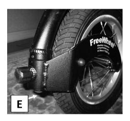
5. Occasionally you may want to put bearing grease on the ball bearing under the front knob (and under the spring).
