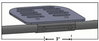
front of tube). Maximum plate angle down is 12 degrees.
