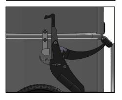
With one hand cupping the clamp of the FreeWheel, hold the clamp to the perch while the other hand grips the handle and firmly close the clamp onto the perch. This takes a little practice.
