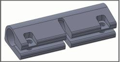
If your TiLite clamp looks like the clamp to the left, this WILL NOT WORK and you will need to order Part P102, which includes a clamp, shim, and pinning screws.
