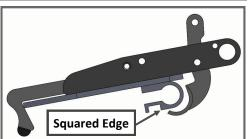
If your TiLite clamp looks like the clamp to the left, with a squared edge at the bottom, you will need to either replace with Part P102 or use a dremel and remove material and curve the bottom (see picture on right).
