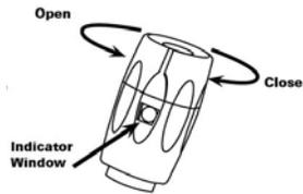
The Pressure Setting Valve (PSV) has 3 numbers shown in the window. The recommended setting of 2 is usually optimal. The internal pressure of the cushion is 0.2 psi and VARILITE® recommends this setting unless otherwise specified by a therapist. See the pressure mapping difference in fully inflated 1, 2, and 3 below.
