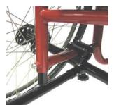
Effective immediately, RGK UK will not be providing raw frames to customers in the future. All units requested that way will be finished as bead blast units. Fifth and sixth wheels on sport products will now look like the image on the left to ensure that the least amount of stress is placed on the camber bars. For those wishing to have rear suspension, it is now
