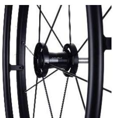
This OMOBIC branded MBL 12 spoke wheel has super potential for the industry with a double wall rim, classic black design, and with only 12 thicker gage spokes. If this wheel was a standard offering on any wheelchair spec sheet it would be a hit! MBL have a plethora of wheels available for the industry, and we stock many of them for same day shipping complete with push rims, tires, tubes, etc.
